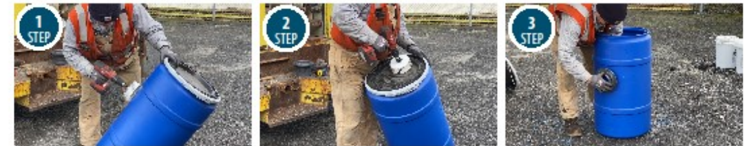
1 STEP Drill a 5-inch hole in barrel in the side of the barrel for a drain. Approximately 18 inches from the top of the barrel.
